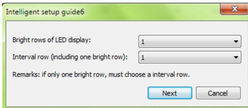
**Interval rows** mean how many black (dim) rows between two bright rows, and then add one bright row for the total interval rows. For example, as shown in below figure, there is one black/dark (mid) row between two bright rows, choose 2 ( $1+1=2$ ) rows for the interval rows, 4 rows for bright row.
