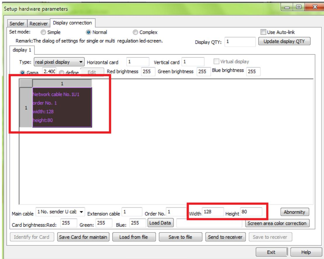
A cabinet with 128\*80 resolution and with two receiving card to support width, the configuration will be as this:
