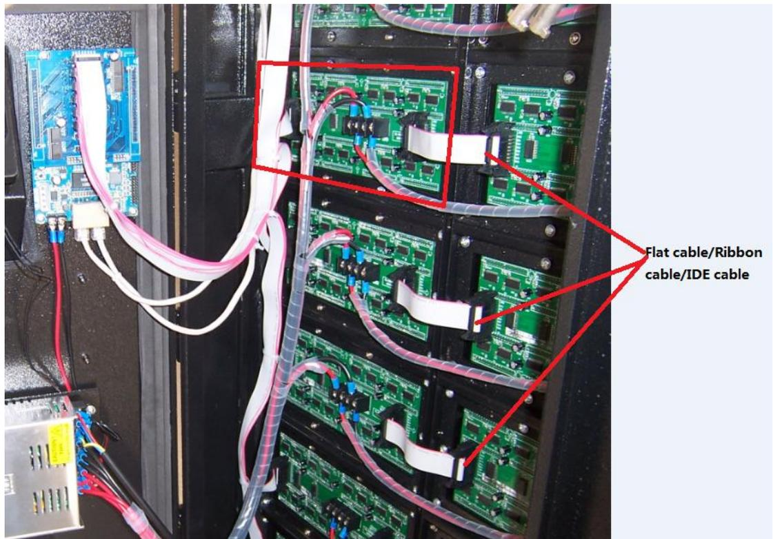
**Data input port:** Input the quantity of the **data input port**, most of the modules are one or two, as above picture it is one data input port (one input port in the left and one output port in the right).
