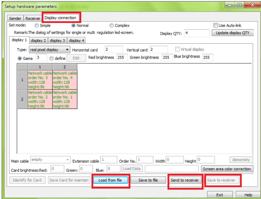
If it is only one cabinet at a time for correction, configure the width and height to be the size of the cabinet. For example: a **cabinet** with 128\*80 resolution, and with **one receiving card**, the configuration will be as this:
